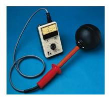
Isotropic Response True RMS Detection 100dB Dynamic Range
